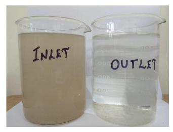
Photo 2.43: Raw waste water and treated water from constructed wetland
