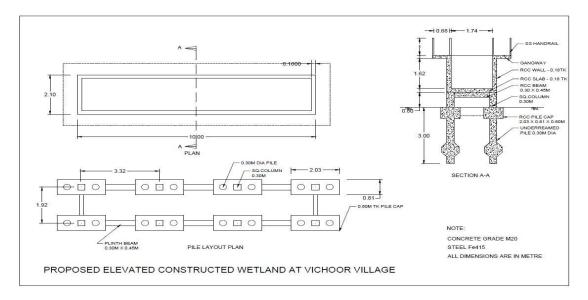
Fig. 3.6: Drawing of elevated constructed wetland
