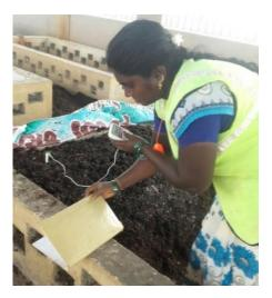
Photo 3.40: Sample collection from compost pits and daily temperature monitoring Table 3.2 Treated water quality from individual treatment plant units
