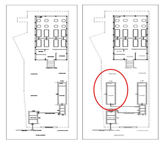
Fig. 3.5: Drawing of elevated constructed wetland at the compost yard
