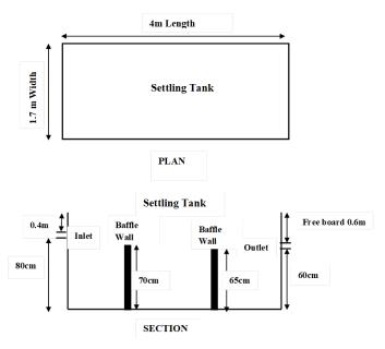
Fig. 2.6: Settling Tank
