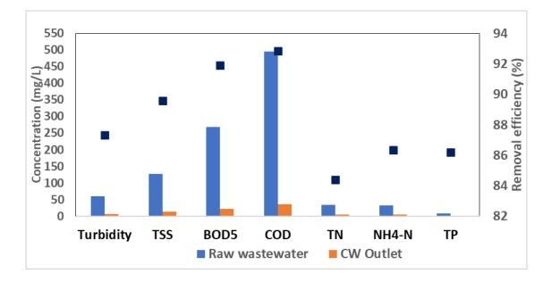
Fig. 3.2: Performance of constructed wetland (after installation of septic tank)
