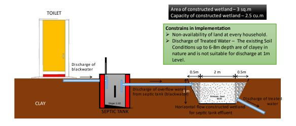
Annexure 5.2 Household Drain Field System for treatment of waste water
