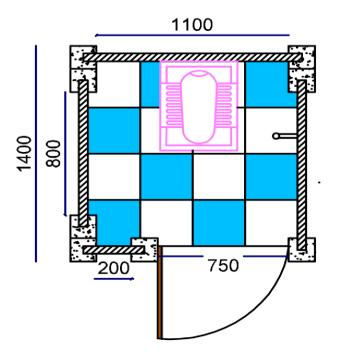
Subsequently the scope widened to attach the bathing facility with overall inner dimension of 4'\*7' size using precast modular structure for walls based on popular demand in consultation with CPCL authorities also. The modified layout is shown below:
