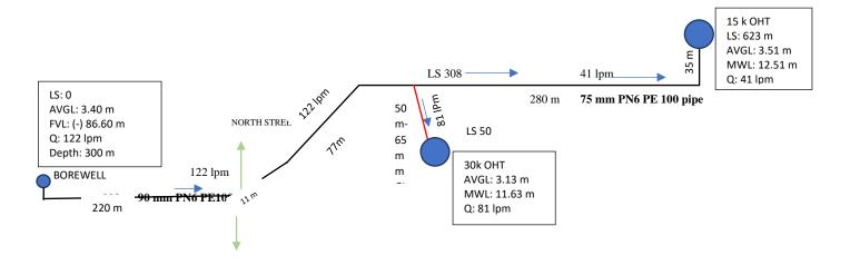
The pipeline provided include the following array of pipes to feed the existing OHTs as shown in the flow diagram above:
