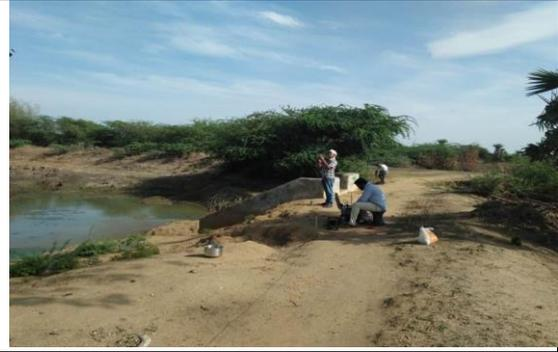
**P1-VES Geo Physical survey to detect desirable Tube well locations**
