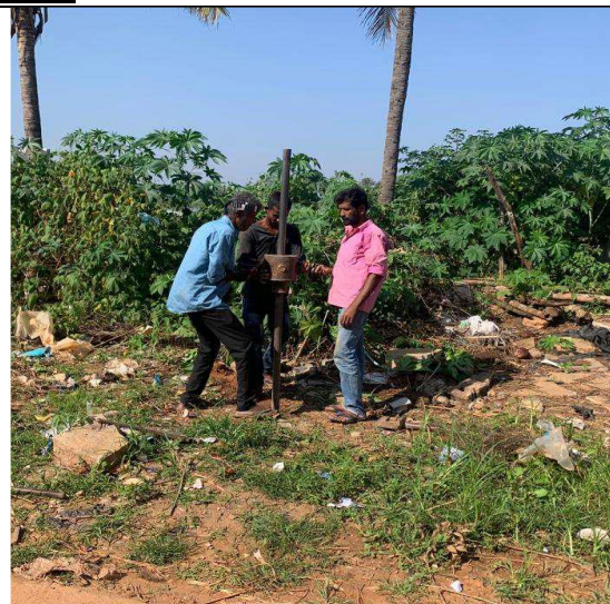
Sample Collection by Boring
